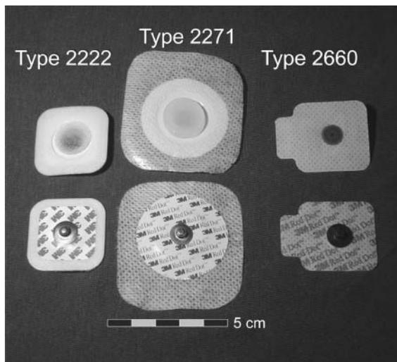
**Fig. 2.** Electrode types used in the study for registration of a multichannel electrogastrogram: the 2 cm<sup>2</sup> conductive area of type 2222 consists of a sponge soaked with a liquid conductive medium, type 2271 has a 3 mm high cylinder made of a firm conductive gel with a 2.54 cm<sup>2</sup> circular conductive basis, whereas the whole 11.64 cm<sup>2</sup> area of type 2660 is layered with a sticky conductive gel.
